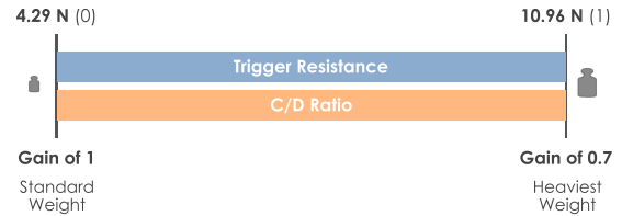
Figure 3: Linear mapping between both stimuli ranges that were applied in our user study. For the analysis, we expressed the magnitude of weight rendering with a normalised value between 0 (standard weight) to 1 (heaviest weight), as indicated by the values in brackets.
