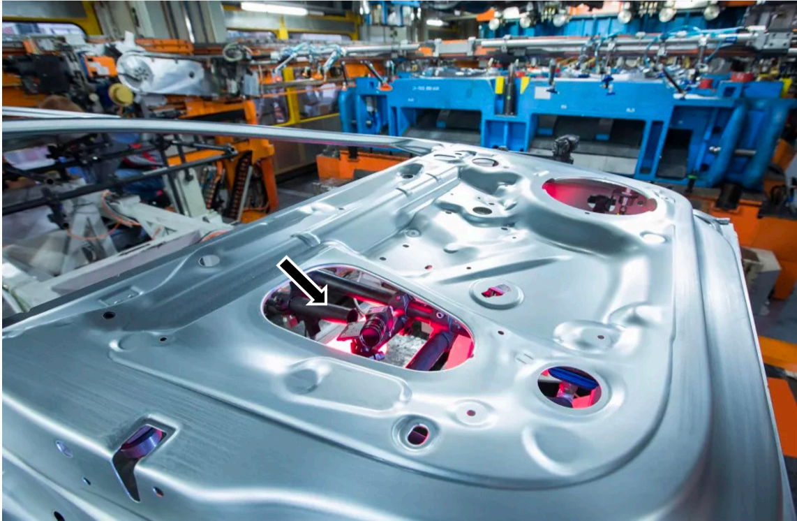
Figure 4: Camera Installed Underneath a Door Side Panel in the Press Line 38
