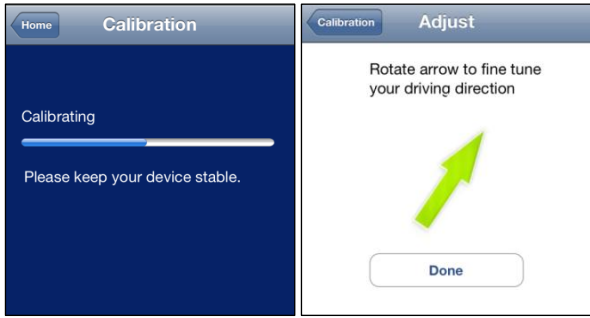
Figure 5. Automated and manual calibration of principal direction of vehicle movement
